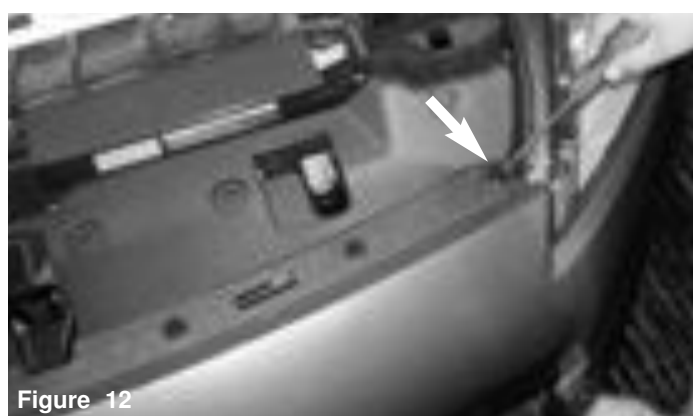
Figure 12 Pop all 7 plastic tabs and remove clips located on the bumper lip.
