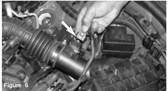
Figure 4 Loosen and remove the 10mm bolt that secures the air box top to the fender.
