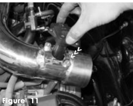
Figure 11 Insert the MAF sensor into the machined intake adapter.
