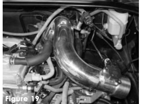
Figure 19 The primary intake is installed and ready for the filter.
