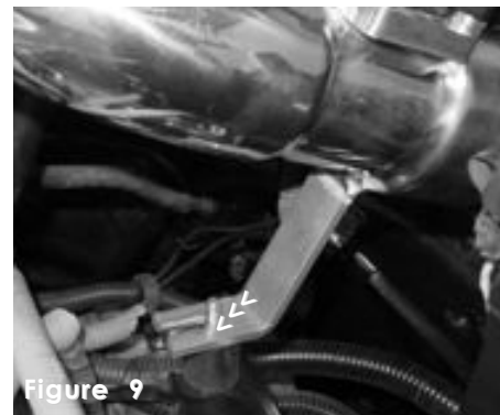
Figure 9 As the upper intake is pressed into the throttle body hose, align the intake bracket to the vibra-mount stud.
