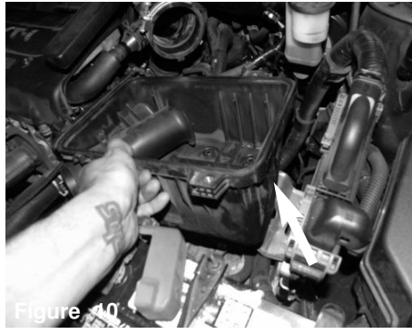
Figure 11 Disconnect crank case line from intake tube fitting.
