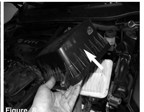
Figure 8 Remove upper half of air box. Remove air filter.
