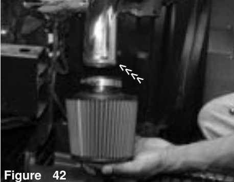
Figure 42 align the filter to the end of the intake located in the bumper area.
