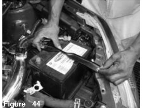
Figure 44 The battery tie down is now placed over the battery to hold it in place.
