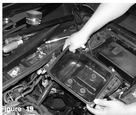
Figure 16 The stock filter panel is removed from the lower air box.
