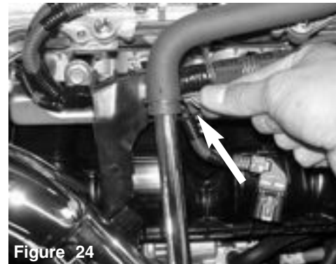
Figure 24 Press the pressure clamp back onto the factory breather line.
