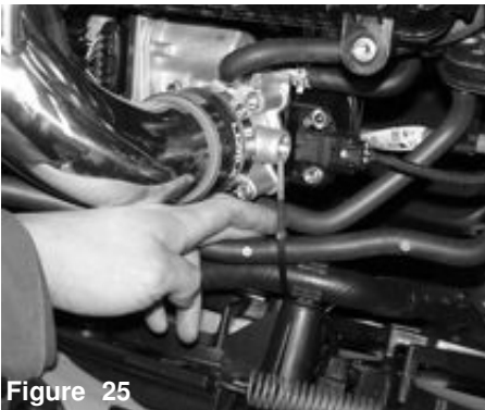
Figure 25 Zip tie the loose coolant line that was originally attached to the factory airbox.
