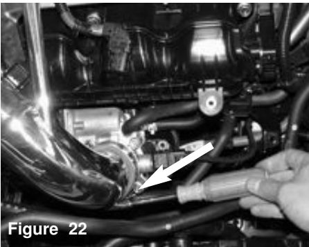
Figure 22 Tighten the second clamp to secure the intake pipe on the 2.5" hose that was already on the throttlebody
