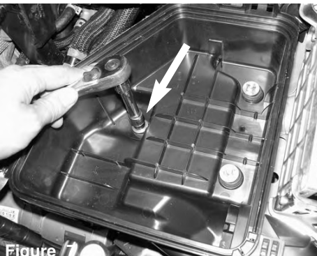
Figure 7 With 10mm socket or wrench, loosen and remove the 3 bolts holding in bottom half of air box.
