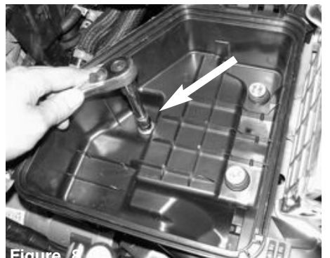
Figure 8 With 10mm socket or wrench, loosen and remove the 3 bolts holding in bottom half of air box.
