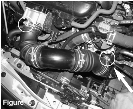
Figure 6 With 10mm socket and wrench, loosen the clamps on the throttle body and the air box.
