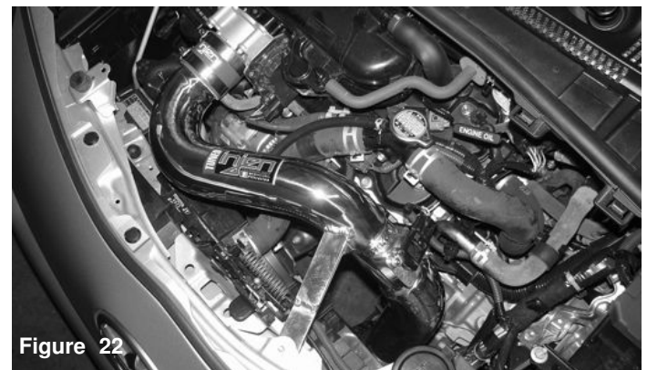
Figure 20 A) Re-connect the MAF sensor harness. B) Attach the crank case line to the fitting on the intake tube.
