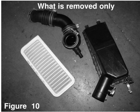
Figure 10 The bottom half of the OEM air box is molded to the radiator shroud. That will stay in place and not be removed.
