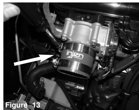
Figure 13 With clamps provided, install the 2-3/8 hose to the throttle body and position. Tighten the clamp on the throttle body only using 8mm nut driver.
