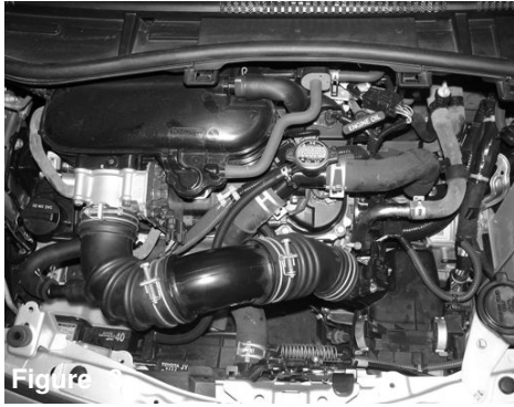
Figure 3 Stock air box shown in this picture.
