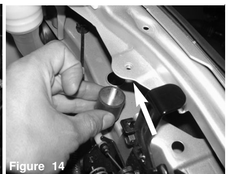
Figure 14 Now install the vibra mount from the bottom up towards the threaded insert located on the radiator support.
