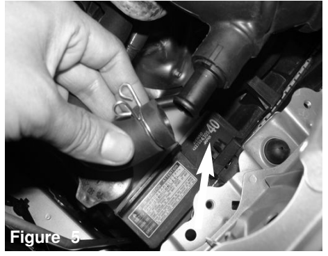
Figure 5 Disconnect the crank case line from the stock intake tube.
