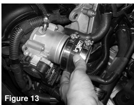
Figure 13 Place the 3.00" straight hose and 2 48 clamps onto the throttle body
