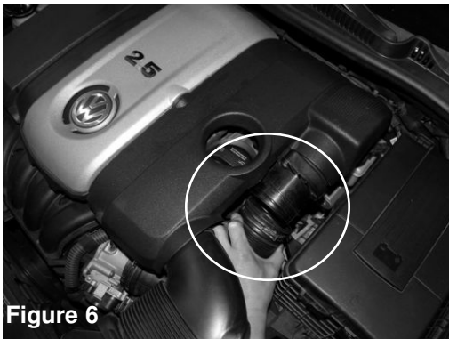
Figure 6 With the pressure clamp loose pull the air duct off the air box
