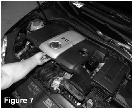
Figure 7 Firmly lift up on the air box/engine cover and remove from the engine bay
