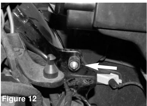
Figure 12 Vibramount shown mounted to chassis
