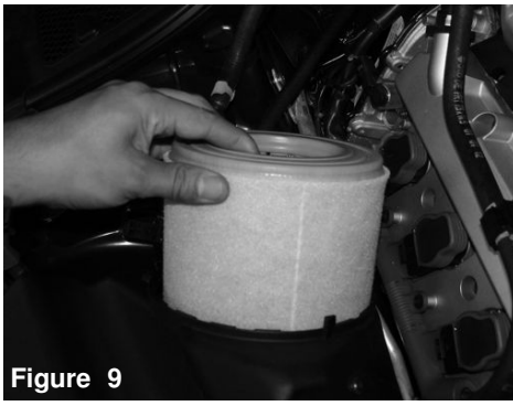
Figure 9 Now remove the filter out of vehicle.
