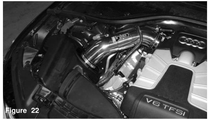
Figure 20 Attach the vacuum line to the fitting located on intake tube and secure.
