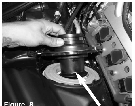
Figure 8 Remove the adaptor out of the vehicle.
