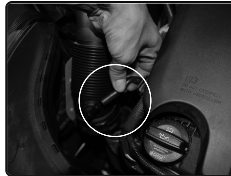
6. Pull back the vacuum line from the OEM intake tube.
