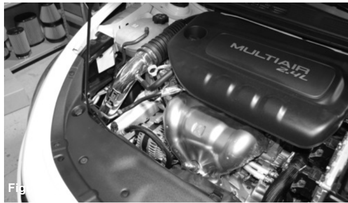
Figure 29 Congratulations! You have just completed the installation of this intake system. Periodically, check the alignment of the intake, normal wear and tear can cause nuts and bolts to come loose. Note: Check clearance and adjust if needed! Failure to check the alignment and adjust the intake can cause damage that will void the warranty. Injen Technology is not responsible for any damages caused by/from improper installation.
