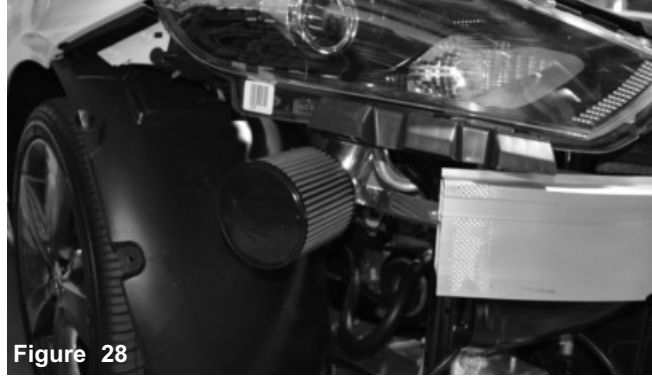
Figure 28 Re-position if necessary and tighten if needed. Make sure there is enough clearance. Re-install the bumper cover and connect the battery terminals.
