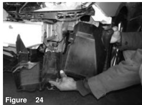
Figure 21 The first m6 bolt is removed from the splash guard.
