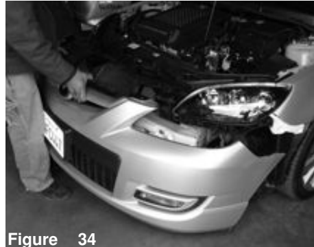
Figure 34 Once you have aligned and tightened all nuts, bolts and clamps, continue to install the front bumper to its original position.
