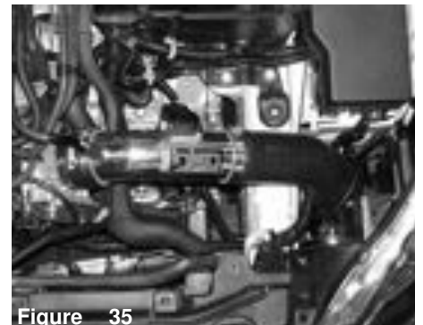
Figure 32 Tighten all clamps on lower intake located on the silicon intake hose (A) Now tighten the clamp on the upper silicone intake using an 8mm nut driver.
