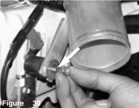
Figure 27 Attach female side of vibra mount to M6 stud on horn bracket.
