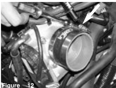
Figure 12 Press the silicon hose with clamps over the throttle body hose. Tighten the clamp over throttle body only using 8mm nut driver.
