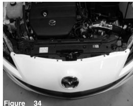
Figure 31 Tighten and secure the intake bracket using 10mm socket and ratchet.
