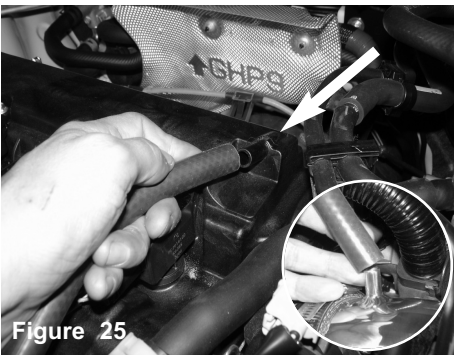
Figure 25 Install the provided new crank case 10mm hose and secure on engine and intake side.
