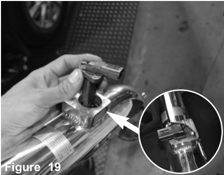
Figure 19 Install the MAF sensor into the intake tube and secure using provided M4 screws. Tighten using 2.5mm allen key.
