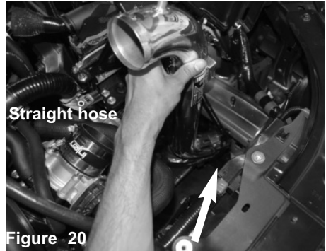
Figure 20 Install the straight hose with clamps to the throttle body. Install the intake tube in to vehicle and position the tube to straight hose and bracket to vibramount from step 17.
