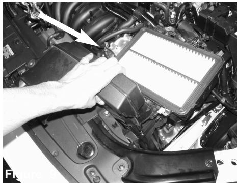
Figure 6 Loosen the clamp on the throttle body using 10mm socket and ratchet. Pull back crankcase line from intake tube.
