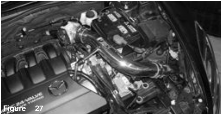
If vehicle was jacked up, lower vehicle. Connect battery terminals. For short ram install, remove the lower intake assembly and place filter on upper intake tube assembly. See figure 28.
