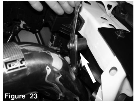
Figure 23 Secure and tighten the bracket using a 10mm socket or wrench.
