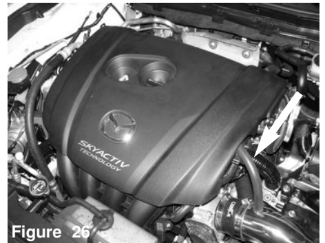
Figure 26 Re-install the engine cover.
