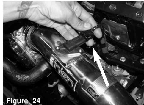
Figure 24 Re-connect MAF sensor harness.
