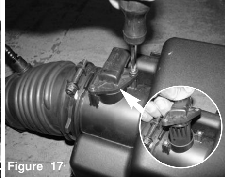
Figure 17 Loosen the screws holding in the MAF sensor. Remove the MAF sensor.
