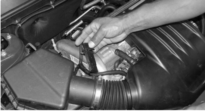
Remove the mass air flow sensor from the stock air intake box. Set the sensor to one side to be used later in the instruction.
