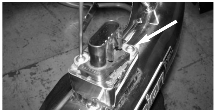
Take the MAF sensor removed earlier from the stock air intake box and press it into the machined adapter. Use the stock sensor screws to reattach the MAF into the machined adapter. Secure the MAF sensor using the 2 M4 screws provided.
