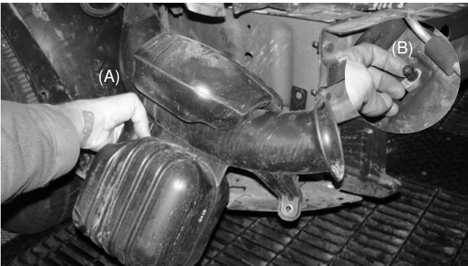
Remove the front bumper cover. With 10mm socket and ratchet, remove the resonator box from the vehicle (A). Remove the air box fitting, this will allow for the vibra mount to be secured (B).
