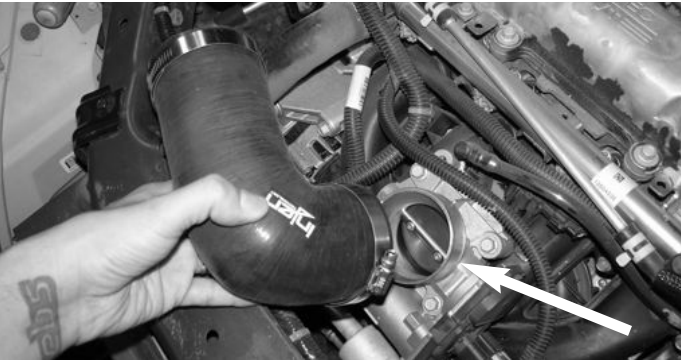
Install the elbow hose with clamps to the throttle body.
