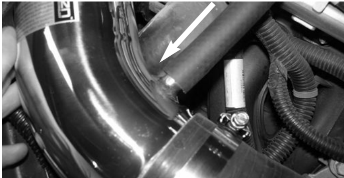
Take the 7" 12mm heat hose and press one end over the crankcase port and the other end over the intake port.
