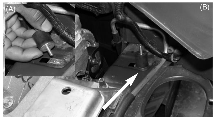
Install the vibra-mount (A). Place the vibra-mount into the pre-tapped hole and turn the vibra-mount into the tapped hole until it bottoms out (B).
