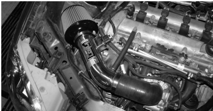
Tighten all clamps using 8mm nut driver. The short ram is now fully installed and ready to go.
