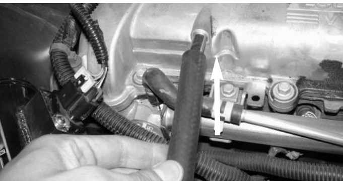
Replace the hose with the new provided 12mm hose .
