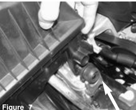
Figure 7 Pull back the front grommet from the bottom of the air box.
