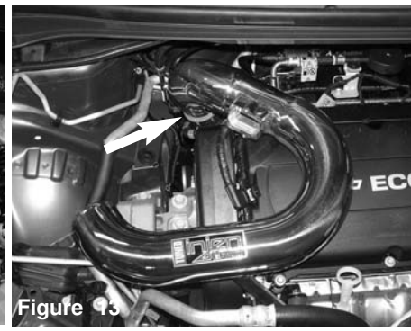
Figure 13 Attach the pipe to the hose located on the throttlebody. Do not secure the clamp for now.
