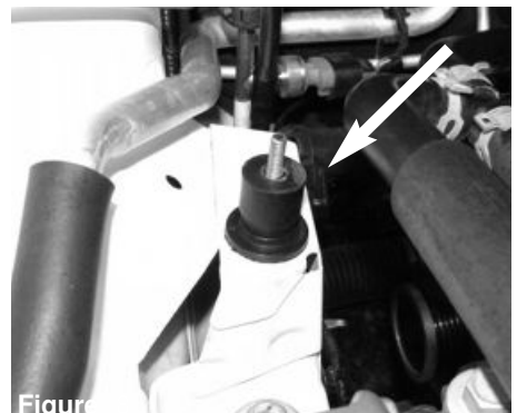
Figure 5 Loosen the clamp on the turbo using 8mm nut driver. Pull the hose away from the turbo housing.
