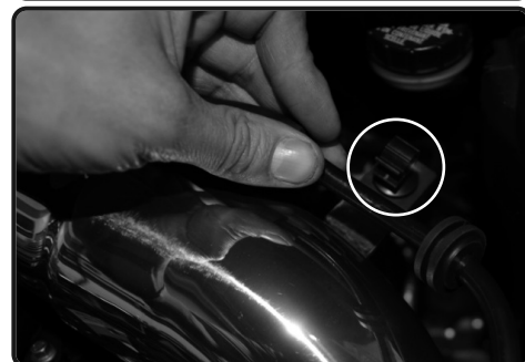
23. Secure the vacuum line to the clip from step 18.
