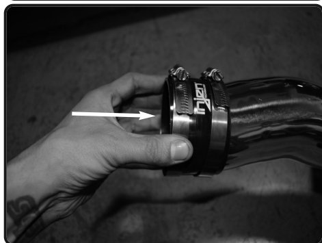
17. Install the 2.25" straight hose with clamps to the intake tube. Do not tighten.
