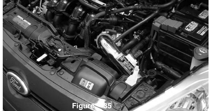
Figure 35 Align the entire intake for the best possible fit. Once you have rechecked and cleared the intake from all moving parts, continue to tighten all nuts, bolts and clamps.
