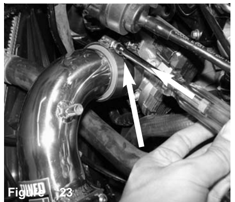
Figure 20 Attach the 2-3/4" straight hose with clamps provided to upper intake tube assembly and tighten on tube only.
