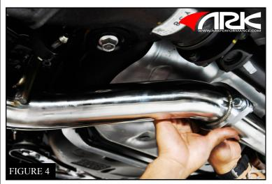
sliding the metal hanger from the mid pipe into it (Figure 4)
