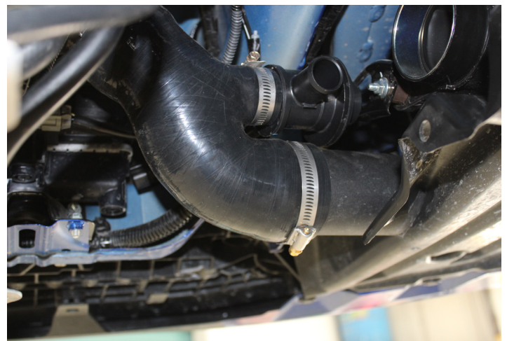
REAR VIEW W/ DIVERTER VALVE:
