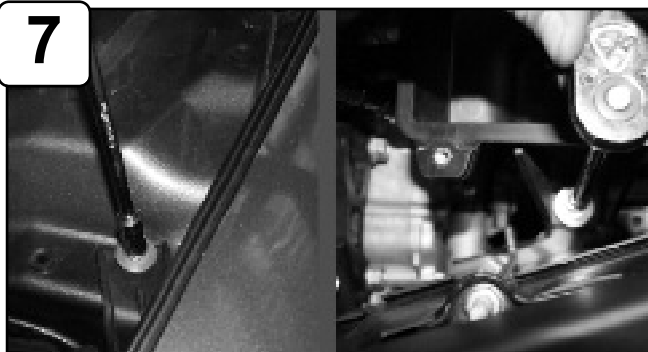
With 10mm socket or wrench loosen both bolts on stock bottom air box and remove.
