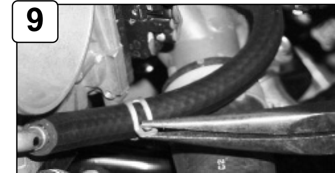
Replace throttle body coolant line with 5/16" hose provided and secure with clamps used from step 8.
