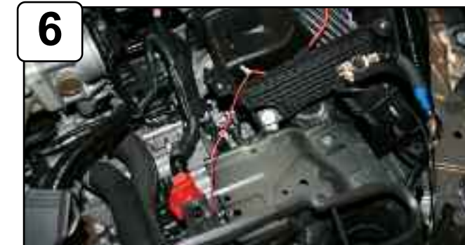
Remove battery out of vehicle.
