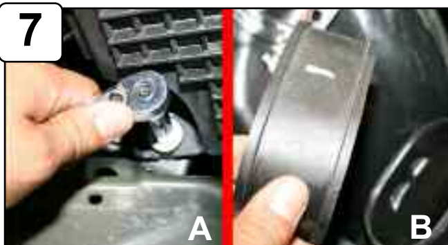
A)With 10mm socket or wrench loosen bolt on stock bottom air box and remove. B)Remove factory coupling.
