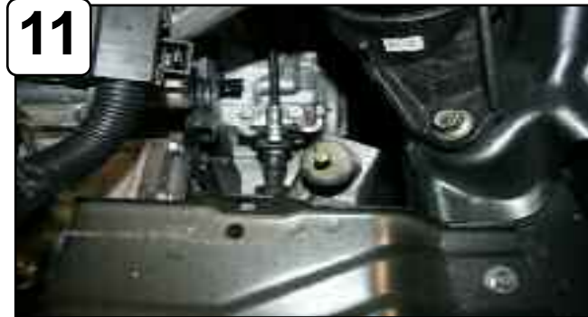
11 Install isolation mount to factory mounting insert next to battery tray.
