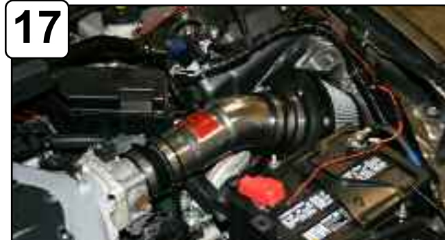
17 Tighten all clamps using 5/16" nut driver. Re-install battery and connect battery terminals. Re-install driver side plastic covers from step 3.
