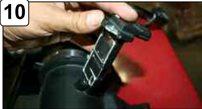
10 Remove MAF sensor from stock air box. Install into new tube and secure using provided M4 screws.
