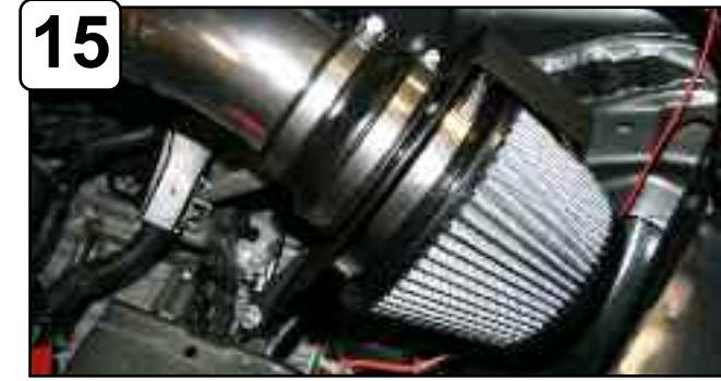
15 Install housing into vehicle and position tab to isolation mount from step 11. Note: Tube may need to be positioned to fit cut out on factory engine cover.
