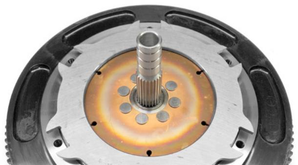
3. Place the final disc onto the flywheel, followed by the pressure plate casting, making sure that the flat friction surface is against the ceramic facing. Ensure the "teeth" of the intermediate plates and pressure plate casting align so that the pressure plate bolt holes are in the gaps, circled in red.
