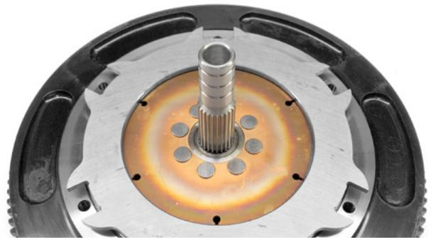
2. Place the second disc onto the flywheel, followed by the second intermediate plate. Note that for quad disc kits, there will be an additional disc & intermediate plate before the final disc and pressure plate casting.
