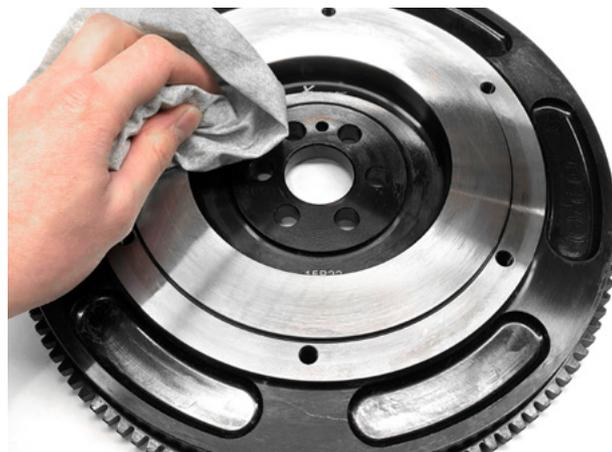
4. If the supplied flywheel bolts do not have pre-applied thread locking compound, manually apply it to the bolts and mount the flywheel to the crank. Torque all flywheel bolts to manufacturers specifications.
