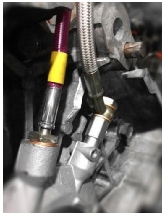
On late model VE II and VF TR6060 transmissions there may be a requirement to remove a small amount of the webbing for a neater route of the line out of the bellhousing hole as illustrated.
