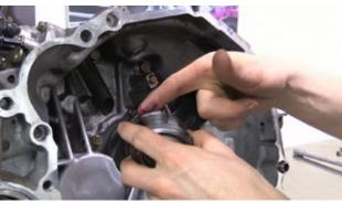
10. Slide the bearing carrier onto the transmission and check for a smooth operation.
