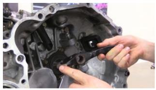
8. Slide the cross shaft in and tighten the retaining bolt.
