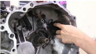
9. Lubricate the contact points on the bearing carrier and snout of the transmission.
