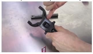
7. Install the clutch fork backwards so that the rounded contact points are facing out of the transmission.
