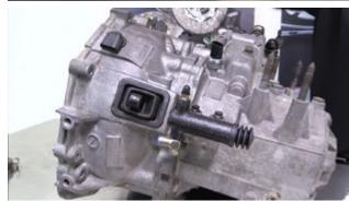
15. Install the new conversion rod over the slave and fork, ensuring that the adjustment bolt is offset towards the top. This will ensure that the rod is not pushing off axis.
