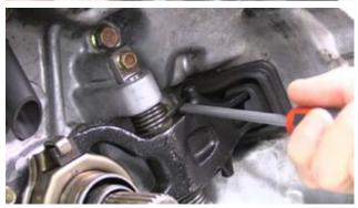
3. Undo the bolt holding the cross shaft in, and remove the shaft.
