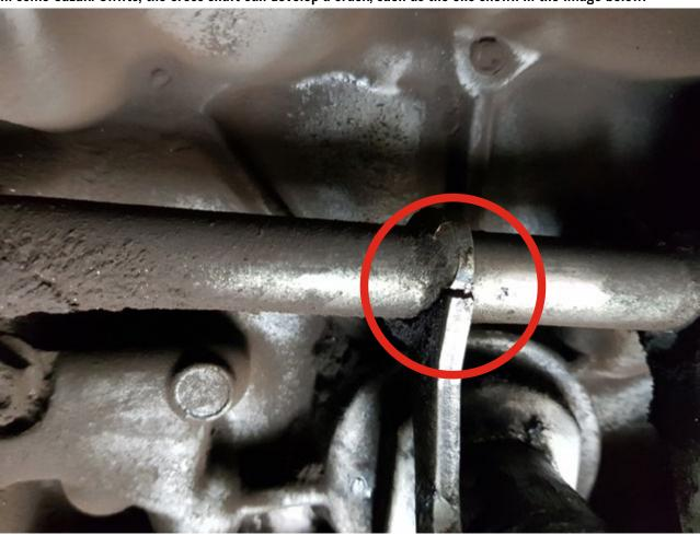
Any damage to the cross shaft can cause the bearing to run off centre and lead to premature wear on the clutch.
