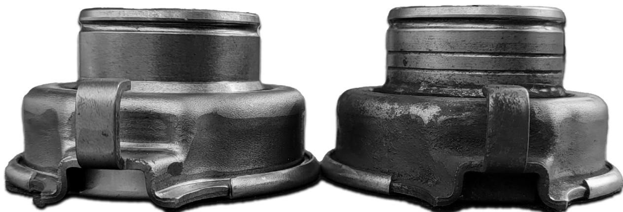
New release bearing (left) compared to OEM Evo X release bearing (right)
