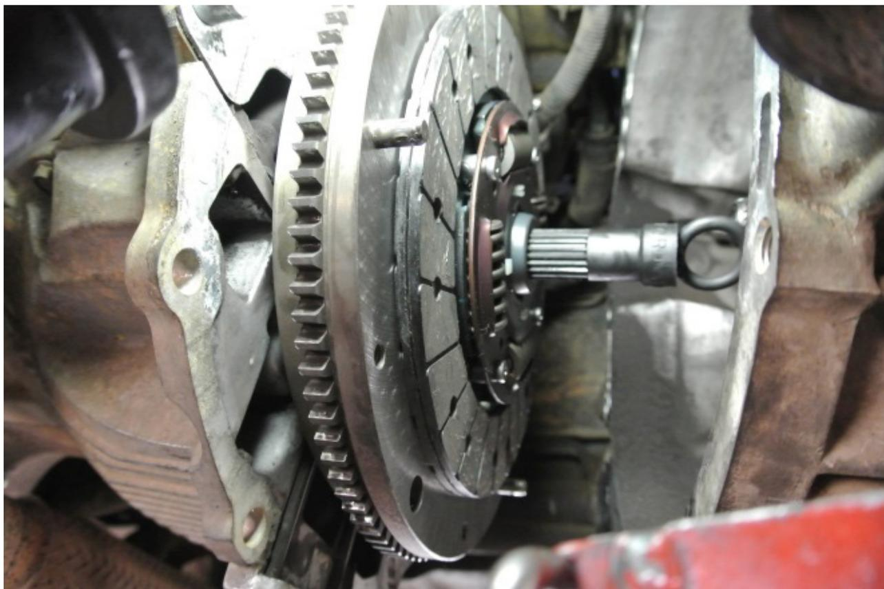
4. Ensure that the pressure plate clip is aligned as per the below photos
