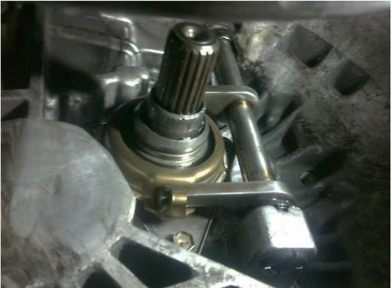
6. Install the release lever onto the release shaft.
