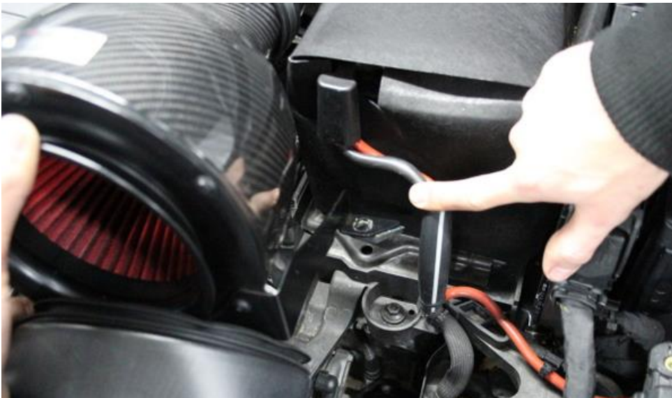
18. Lower the housing – push the battery cables away to allow the bracket to lower into position.
