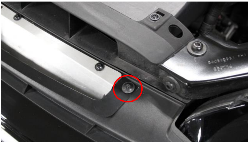
36. Secure this side too – the screw should go through the scoop surround.
