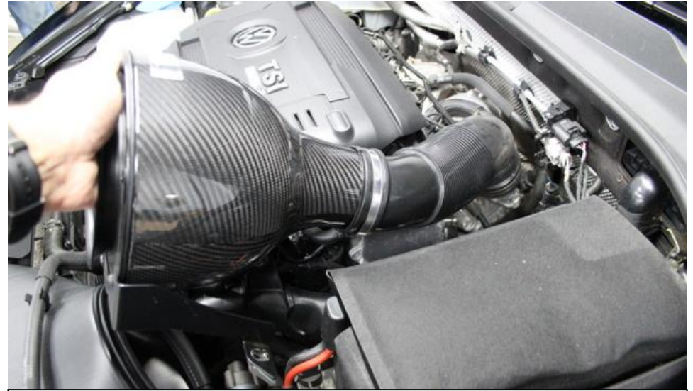
17. Now take the filter housing and push into the stock tube fully. The Eventuri badge should be on the top of the housing for correct orientation.
