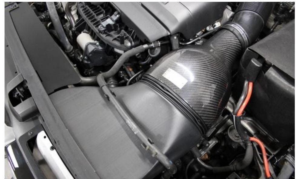
19. Lower the housing so that it locates inside the duct as shown. The rubber seal should be evenly compressed.
