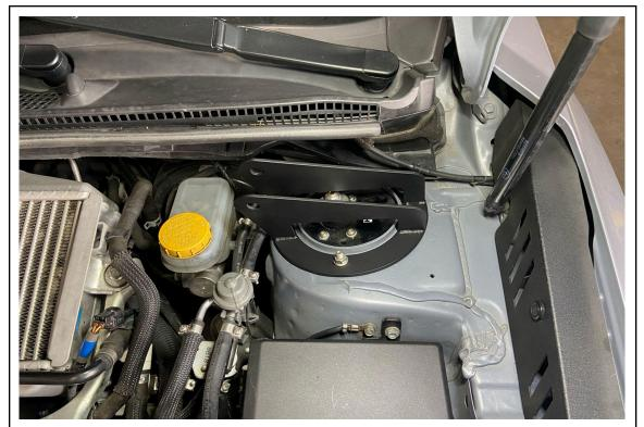
5. Loosely install bracket 431-116-L onto the driver side strut tower using the factory nuts removed in step three.
