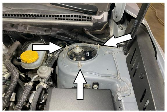
3. Remove the three nuts from the driver side strut tower and set aside.
