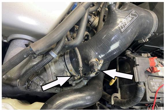
5. Connect the HPS intake tube to the throttle body and secure it with the provided EMSC-70-90 clamp. Push the air temperature sensor into the HPS intake tube and secure it using the provided EMSC-12-22 clamp.
