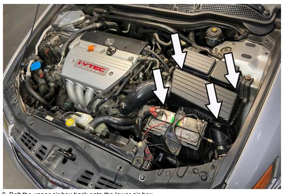
6. Bolt the upper air box back onto the lower air box.
