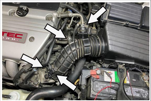
3. Disconnect the breather tube and the idle air hose from the intake tube. Next, remove the air temperature sensor from the intake tube and loosen the hose clamp securing the intake tube to the throttle body. Remove the intake tube along with the upper air box from the vehicle.
