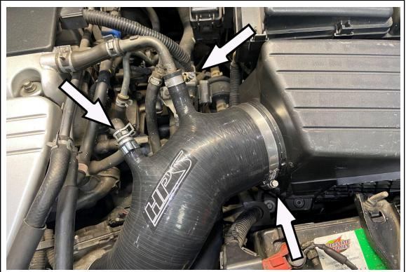
4. Connect the HPS intake tube to the upper air box using the provided EMSC-80-100 clamp and place the HPS intake tube and upper air box back into the vehicle. Push the breather tube into the HPS intake hose and secure it using the EMSC-16-27 clamp. Connect the idle air hose to the HPS intake barb and secure it with the factory clamp.
