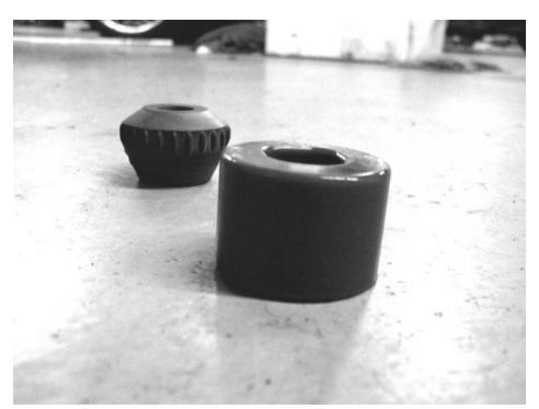
5 . Remove the original foam rubber engine mount and replace it with the APR Polyure-thane Snub mount. The APR snub may require some force to press onto the aluminum engine mount (silicon grease or soapy water will help)
