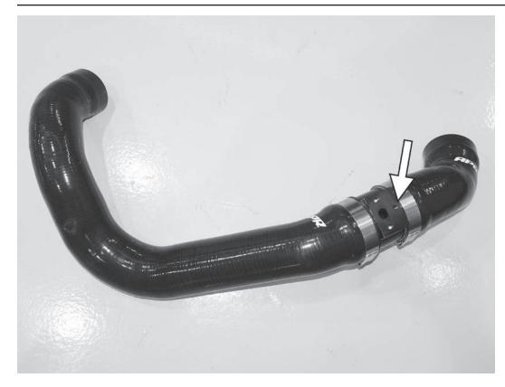
35) Loosely assemble the shown hose assembly using the APR MAP housing, APR hose Z1003201, APR hose Z1003202, and two 3" (-0300) hose clamps. The single small screwhole on the top of the APR MAP housing should face the shorter hose.
