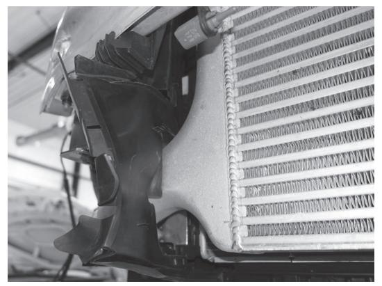
33) Reinstall the right plastic air guide that runs up and down the right, front side of the radiator and intercooler. The guide will snap back into the original mounting points from where it was removed. Also reconnect the lower portion of the left air guide that was disconnected.
