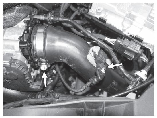
21) Loosen the hose clamp from the stock inlet pipe to the throttle body. Disconnect the electrical connector to the MAP sensor mounted in the stock inlet pipe. Remove the inter-cooler to throttle body hose from the car by carefully pulling the hose down and out from the bottom side of the car.
