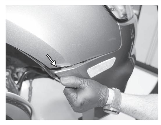
13) Pull both right and left edges of the bumper cover away from the sides of the front fenders.
