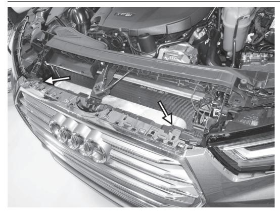
45) Place the bumper cover back on the car. Make sure the tabs on the top of the bumper go into the slots on the top of the bumper support.
