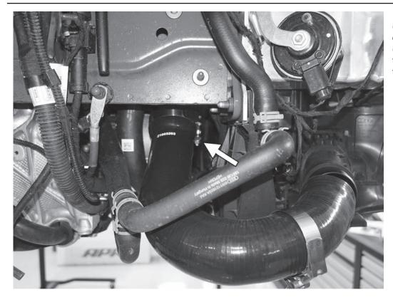
19) Loosely place one of the 3" (-0300) hose clamps on the end of the right APR intercooler hose (Z1003203) and install the hose onto the turbocharger outlet pipe. Do not tighten the clamp yet.
