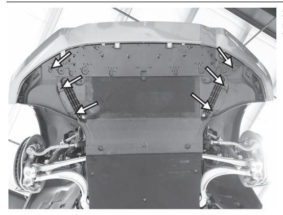
5) Disconnect the four quarter turn T25 screws and two T25 screws holding the lower wheel well liners to the engine belly pan.
