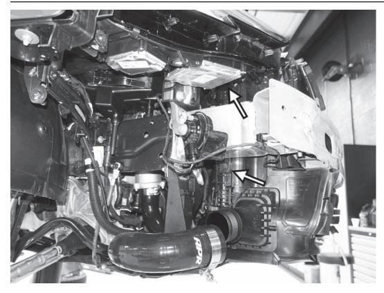
23) Remove the right plastic air guide that runs up and down the right, front side of the factory radiator and intercooler. Push in on the two tabs where the air guide connects to the radiator core support, pull the air guide forward, and then manipulate the air guide out of the car.
