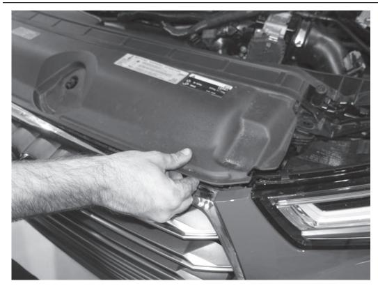
11) Lift up on the front of the upper bumper cover to separate from the bumper, and then pull forward to remove from the car.
