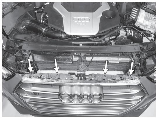
47) Install the four T30 screws holding the top of the bumper cover to the bumper latch support.
