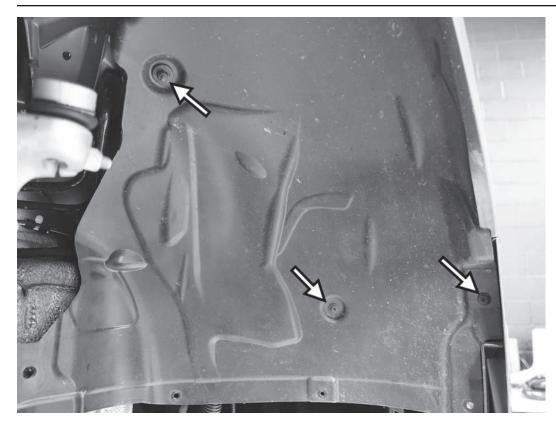
51) On both sides of the car, install the two T25 screws and one 10mm nut holding the front of the wheel well liner in place.
