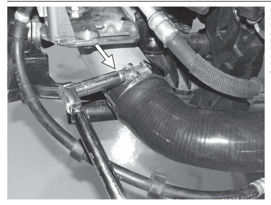
39) Loosely place the remaining 2.75" (-0275) hose clamp on the bottom of the hose assembly, at the APR intercooler outlet. Reinstall the hose assembly in the car, attach the assembly to the intercooler outlet and secure the clamp. Tighten the hose clamp to 50 in-lbs (5.7Nm), but do NOT overtighten.
