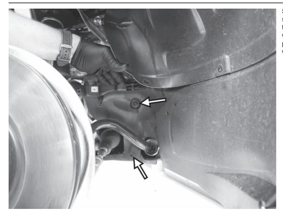
53) On both sides of the car, reinstall the plastic push pin barbed fitting from the upper, inner side of the wheel well liner. Also install the T30 plastic screw from the lower wheel well liner.
