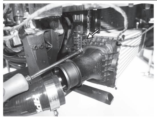
25) Squeeze the release clip holding the right side of the intercooler to the core support, and then carefully use a screwdriver to pry the top of the stock intercooler forward. Repeat on the left side of the intercooler.
