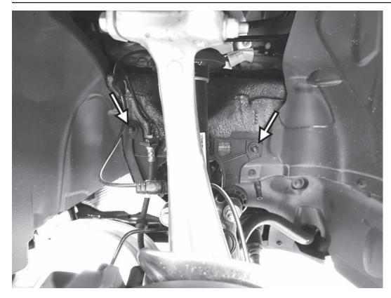
57) Reinstall the plastic axle shield to both sides of the car, and secure with the two 10mm plastic nuts.
