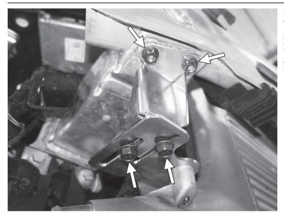
31) Install the upper portion of the APR brackets as shown. The stock 13mm bolts go through the upper portion of the APR bracket and are secured with the factory 13mm nuts. The lower APR bracket and upper APR bracket are connected with the supplied 13mm nuts.
