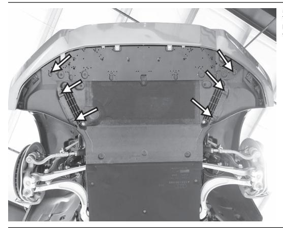
55) Reinstall the four quarter turn T25 screws and the two T25 screws holding the lower wheel well liners to the engine belly pan.
