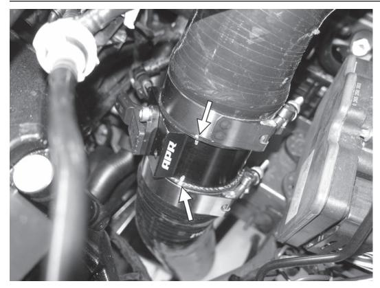
37) Install the APR hose assembly into the car, connecting to both the throttle body and APR intercooler outlet. Manipulate the hoses about the APR MAP housing until you get an ideal fitiment. Make sure the MAP sensor can be connected to its harness without interferance. Once the hoses are rotated correctly, mark the orientation of hoses and the MAP housing using a sharpie or paint marker.
