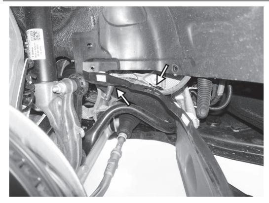
7) On both sides of the car, separate the drain line from the lower wheel well liner and remove the liner from the car.
