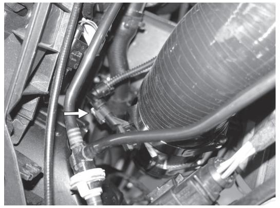
41) Reconnect the electrical connector to the factory MAP sensor, and lock the tab on the connector.
