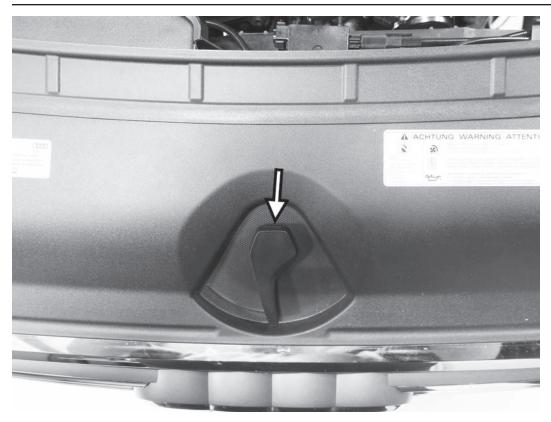
49) Reinstall the hood latch by simply pushing the keyed latch down on the keyed post for the hood latch assembly.
