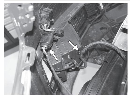
43) With an assistant, bring the front bumper cover back to the car. On both sides of the car, reconnect the wiring harnesses for the ACC radar sensors. Reattach the clips for the harness to the bumper cover, and reconnect the electrical connectors to the park distance sensors.
