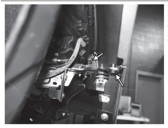
9) After carefully folding back the front of the wheel well liner, remove the T30 screw holding the front of the fender to the back of the bumper cover. Also remove the plastic pushpin clip from between the fender and bumper cover. Repeat on both front wheel wells.
