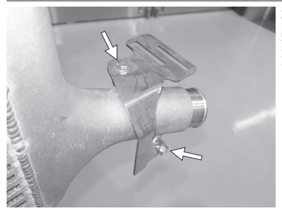
27) Install the two APR lower brackets to the APR intercooler as shown. Use the longer two of the four supplied 13mm screws with a washer in the two lower mounting holes, and use the two shorter 13mm screws in the upper holes. The other side is the mirror of the side shown.
