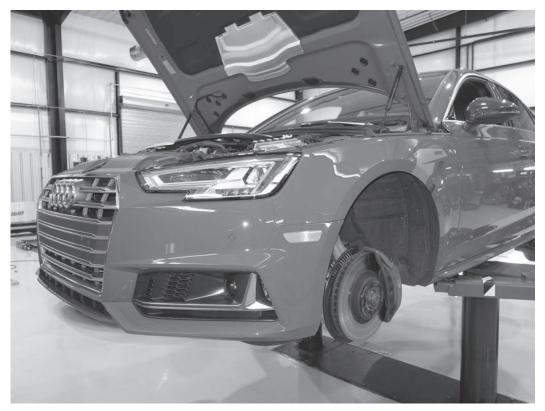
1) Place the vehicle securely on jack stands or on a lift, remove the front wheels, and raise the hood of the vehicle.
