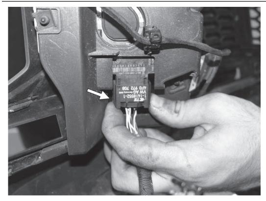
15) Disconnect the electrical connector from both ACC radar sensors. Again, do not turn the ignition on in the car with these sensors unplugged.
