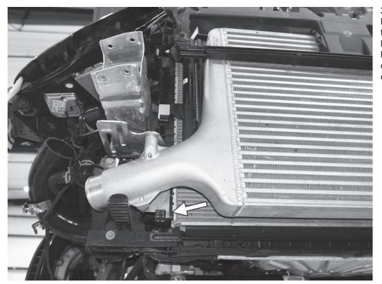
29) Slide the APR intercooler up and behind the upper bumper support of the radiator core support. Set the lower tabs from the APR intercooler brackets down in the tabs that were originally supporting the stock intercooler.
