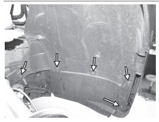
3) On both sides of the car, remove the five T25 screws from the lower section of the wheel well liner.
