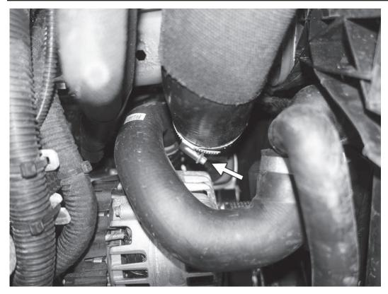
17) Loosen the hose clamp from the stock turbo outlet pipe to the intercooler inlet hose.
