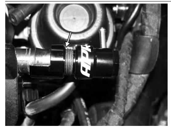
9) Begin to thread the main body of the APR boost tap into the base of the boost tap.
