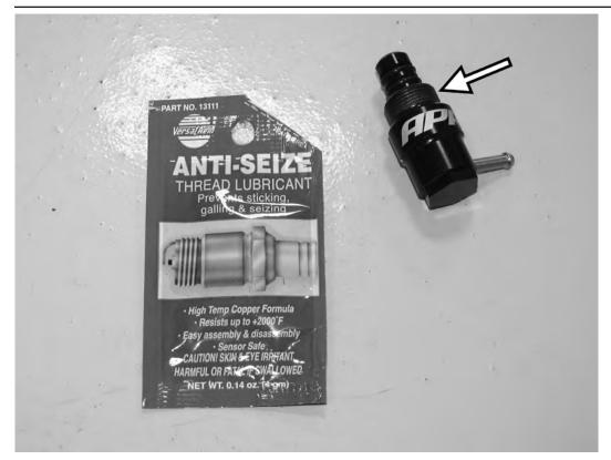
7) Unscrew the two portions of the APR boost tap. Apply a very small amount of the supplied anti-sieze to the threaded portion of the main body of the APR boost tap.
