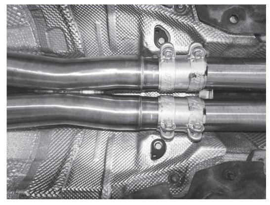
5) Connect the back of the X-Pipe to the now cut section of the APR catback with sleeve clamps. Slide the sleeve clamps in place as shown and very loosely secure them. Ensure the pipes can still rotate inside the clamps for now. There should be approximately a 10mm (3/8") gap between the back of the X-Pipe and the beginning of the APR catback - do not butt the X-Pipe up to the beginning of the APR catback.
