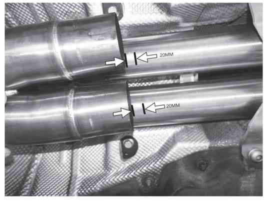
3) Place the X-Pipe underneath the car with the APR midpipes and APR catback already fitted. Align the front of the X-Pipe with the previously made marks that are 90mm behind the catalyst. Then, mark the APR catback approximately 20mm behind the "end" of the X-Pipe.
