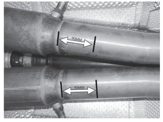
1) With the APR midpipes and catback still installed on the car, make a mark approximately 90mm behind the back of the catalysts, behind the secondary oxygen sensors.
