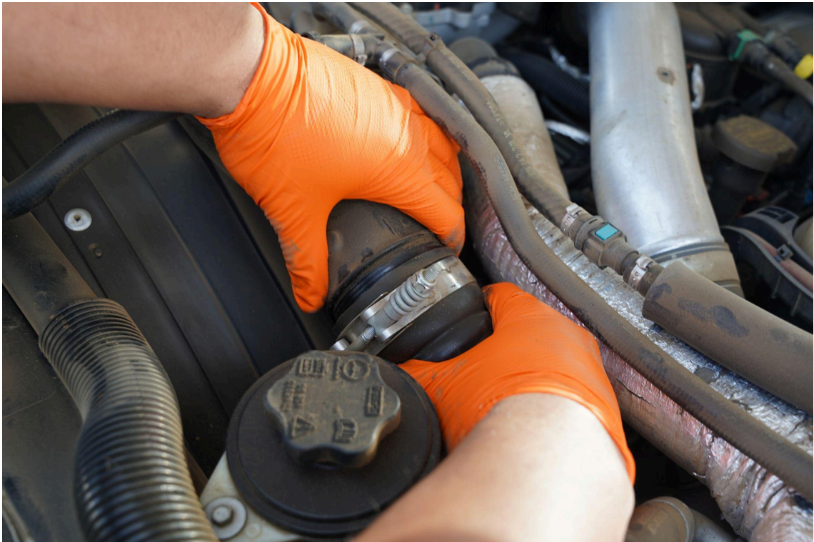
5. Disconnect the factory charge hose from the plastic quick-connect pipe.
