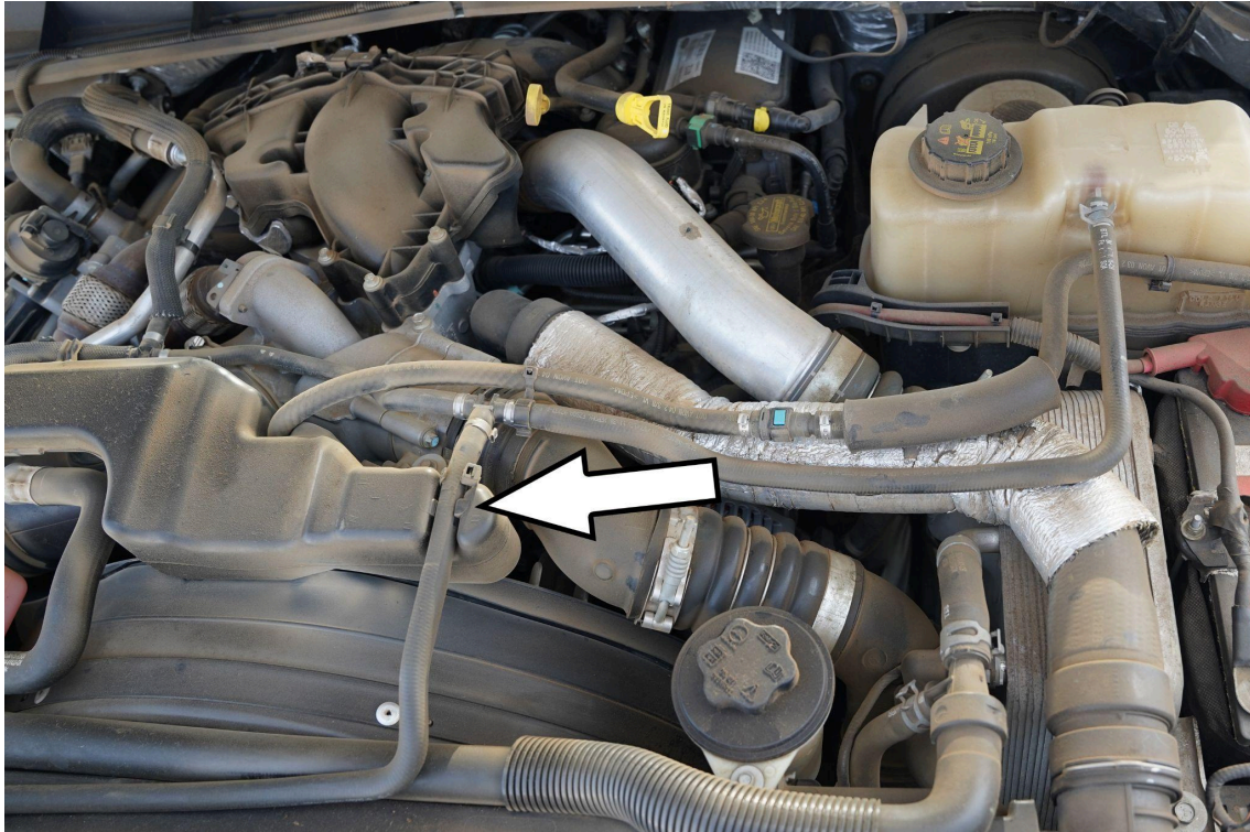
3. Unclip the coolant hose from the resonator mount in order to gain access to the upper quick-connect pipe.
