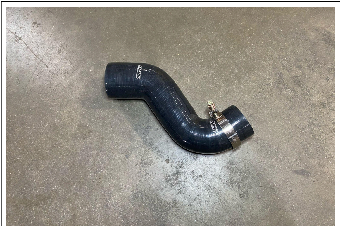
11. Slip provided spring loaded T-bolt clamp onto the 90 degree end of the HPS charge hose.
