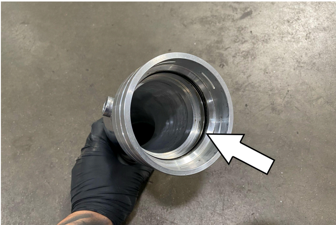
10. Place the provided O-ring into the groove on the HPS charge pipe.
