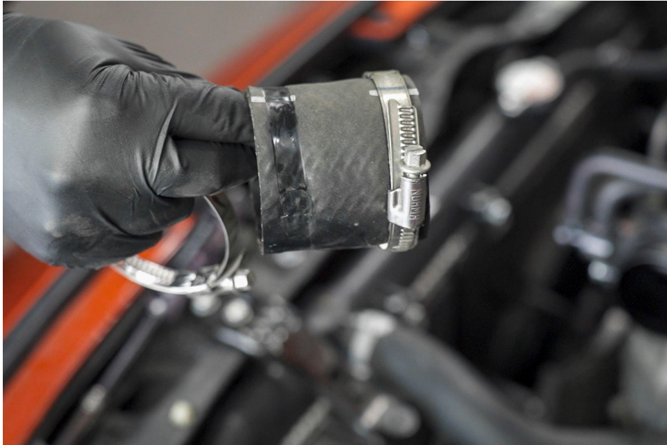
13. Loosen the hose clamp to remove the throttle body coupler.
