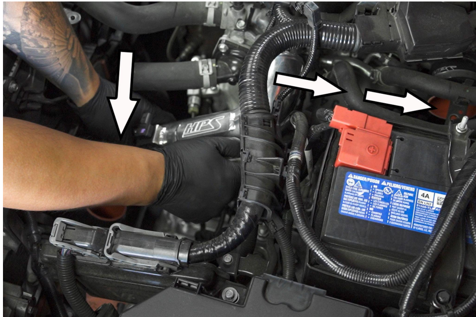
18. Slide the HPS charge pipe down towards the bottom of the engine bay, and then, towards the throttle body. Once the pipe is in position, connect the charge pipe to the reducer coupler, then to the throttle body coupler.
