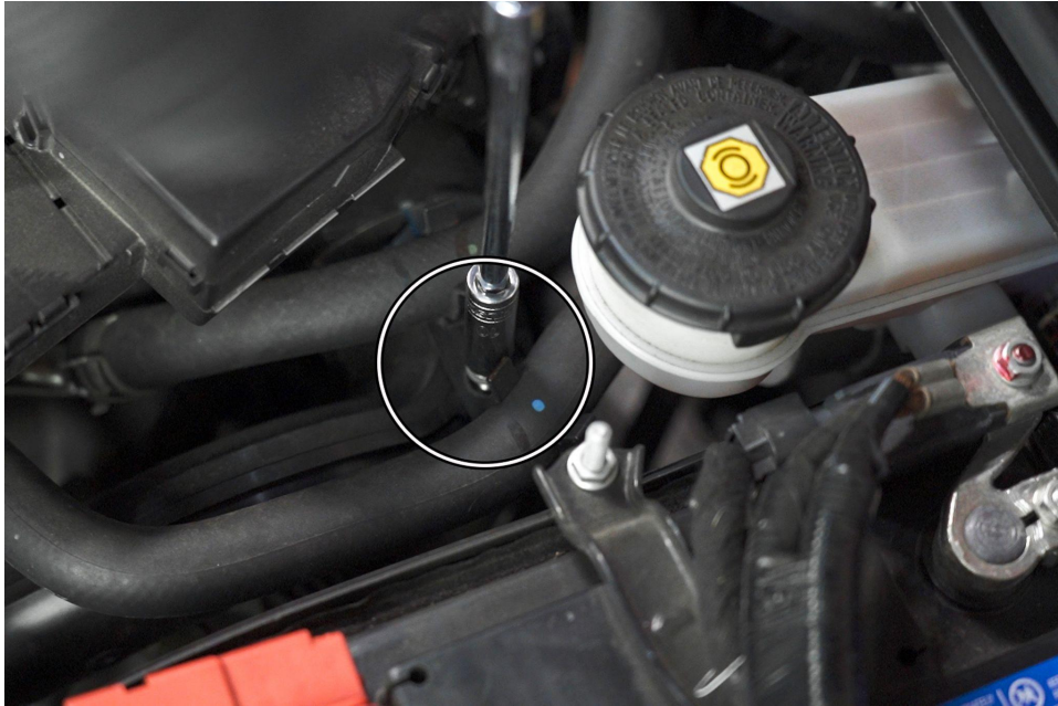
9. Remove the 10mm bolt securing the heater hose bracket from the charge pipe.
