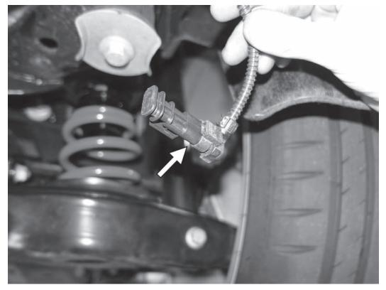
9) Install the dummy connector from the APR harness onto the factory harness that was connected to the exhaust flap motor.
