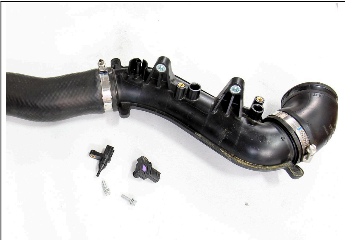
17. Use an 8mm socket to remove the IAT and MAP sensors from the factory charge pipe.
