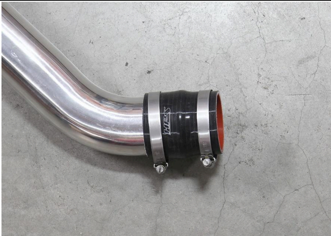
19. Loosely attach the silicone reducer onto the opposite end of the charge pipe as shown.
