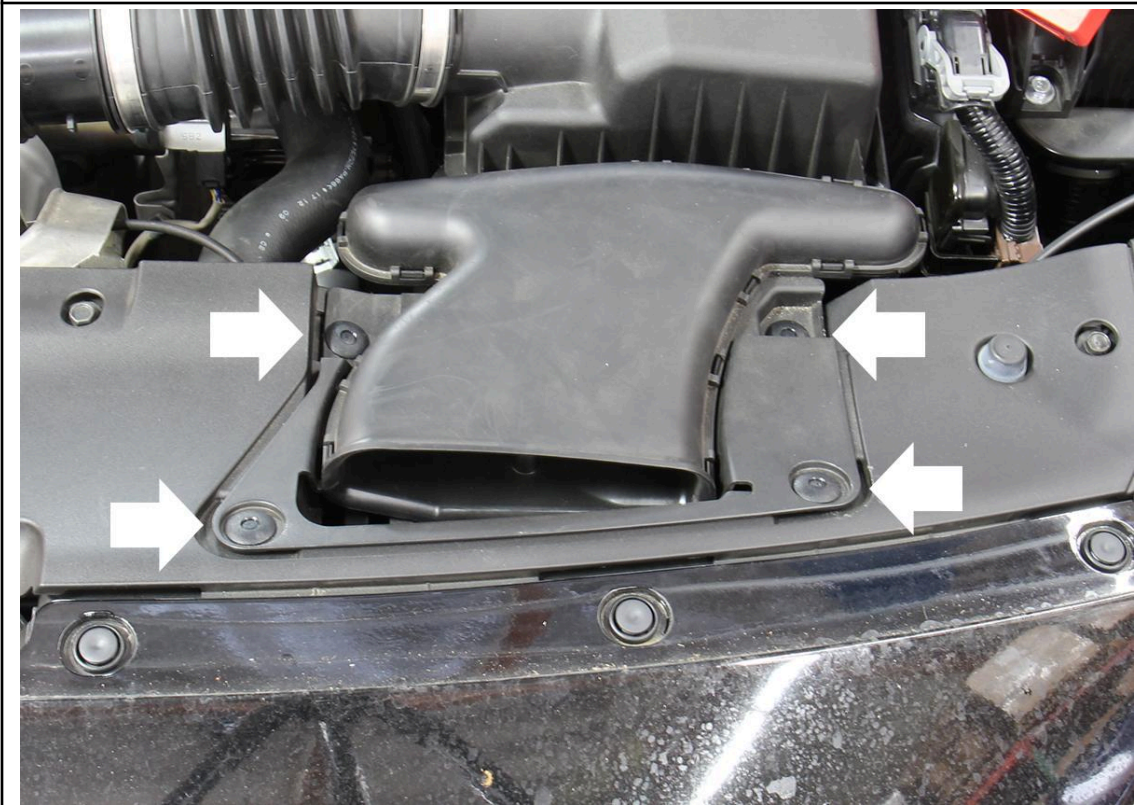
6. Push down at the center of the 4 button clips to remove the air duct from the engine bay.
