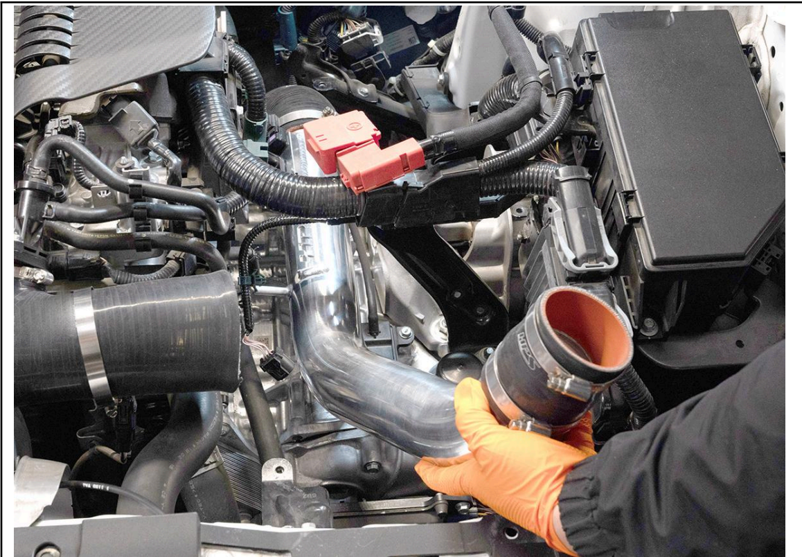
21. Carefully slide the HPS charge pipe into position from the front of the vehicle. Be mindful of objects around the engine bay that may scratch or damage the pipe.
