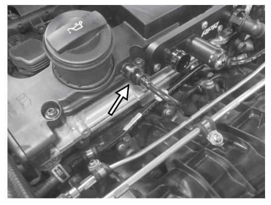
9) Disconnect the vacuum line just to the right of the APR PCV plate on the engine valve cover.
