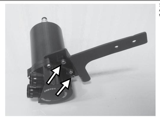
7) Install the APR bracket to the APR catch can as shown with the supplied 4mm allen screws.
