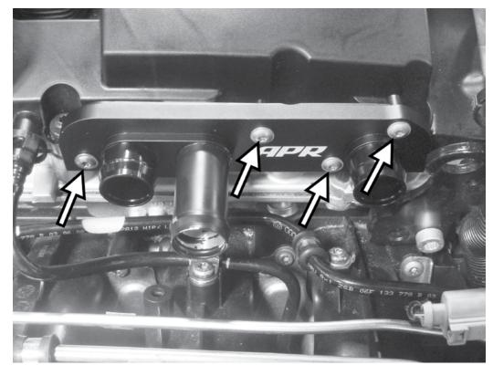
5) Install the APR PCV plate to the front of the valve cover with the four original T25 screws that held the factory PCV in place. Torque these screws to 4Nm (35 in-lb).
