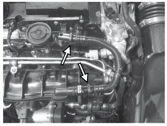
1) Remove the stock hose that goes between the factory PCV valve and the port on the intake manifold by squeezing on the Norma connections to release them. Once removed, install the plug supplied with the APR boost tap in the boost tap with thread sealant to close off this port on the intake manifold.
