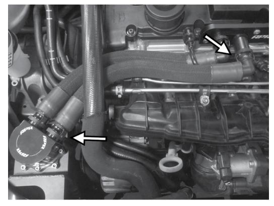
11) Install the other APR catch can hose to the last remaining port on the APR PCV plate, and connect to the last remaining port on the APR catch can.
