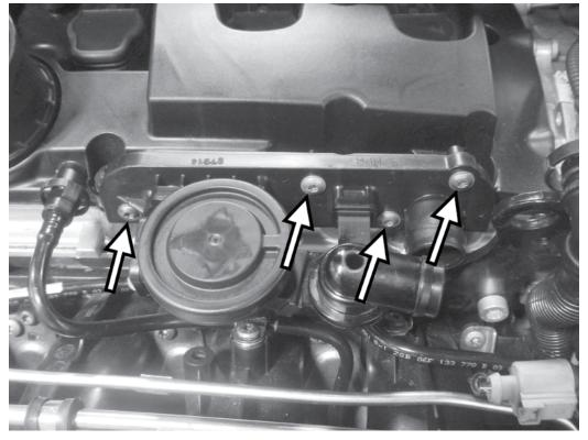
3) Remove the four T25 screws holding the PCV valve to the engine valve cover, and remove the PCV valve from the engine.
