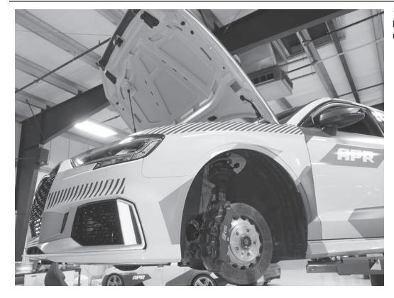
1) Securely lift the car using an auto lift or a jack and jackstands, and remove the front wheels.
