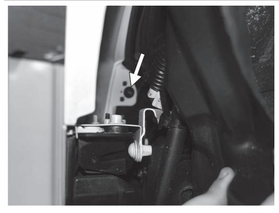
7) Pull back the fender liner and look towards the front of the car from the wheel well. Remove the two T30 screws (one on either side of the car) holding the back of the bumper cover to the front of the fender. The TT-RS does not have this screw.
