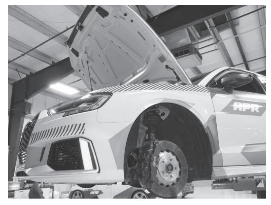
45) Reinstall the front wheels and torque the lug bolts to 88 ft-lbs (120Nm). Take car off lift or jackstands.
