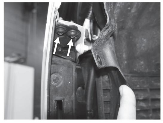
5) Pull back the front of the fender liner and remove the four (two on each side) T30 screws holding the bumper cover to the bottom of the front fender. The TT-RS only has one screw in this location.
